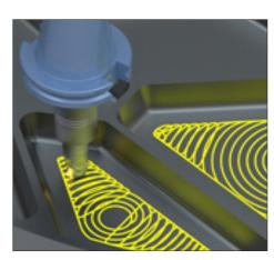
Edgecam Waveform roughing strategy is a high speed machining technique that maintains a constant tool cutting load by ensuring the tool engagement into the material is consistent.
