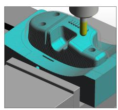
Edgecam Milling provides functionality to program wire frame geometry or solid model component parts on a variety of machine tool configurations, from 2.5 axis milling to complex surface tool paths on 3 to 5 axis milling machines.
