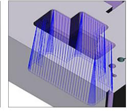
Edgecam Wire EDM provides the flexibility and confidence to manufacture 2 and 4 axis parts accurately and efficiently; providing the ability to easily program complex shapes with irregular tapers.
